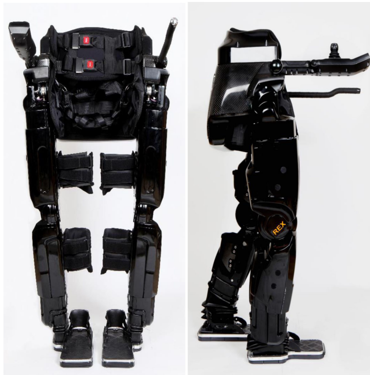
Fig. 1 REX robotic exoskeleton seen from the front and side
